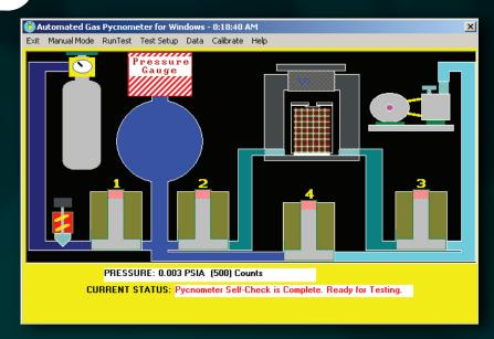
Thus, the true volume obtained by pycnometry includes any pore volume accessible to the gas. Helium is the preferred gas, because it exhibits ideal gas behavior. However, almost any non-corrosive gas including air can be used. The true density is obtained by dividing the weight of the sample by true volume.
